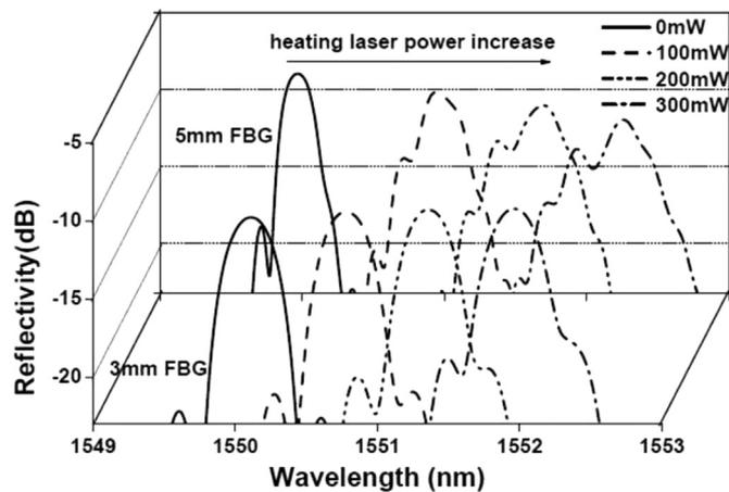
**Fig. 3.** The reflection spectra distortion of the FBGs with different grating length and heated at different heating power levels (experiment results). (a) 3 mm FBG, (b) 5 mm FBG heated using 0 mW, 100 mW, 200 mW and 300 mW heating laser, respectively.
