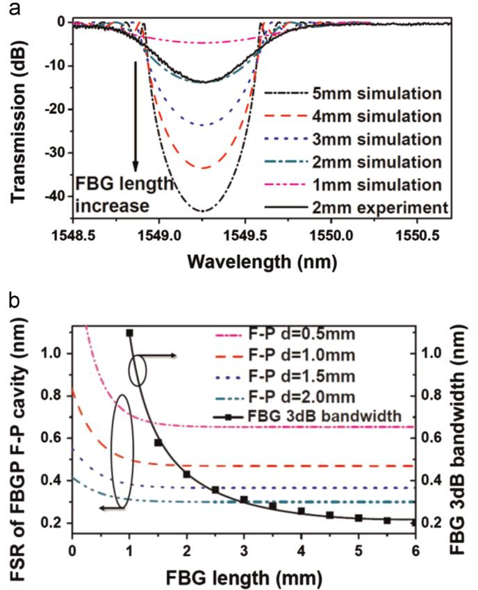
Fig. 2. The FSR of the FBGP formed F–P cavity compares with the bandwidth of the FBGs which form the F–P cavity. (a) Measured and simulated FBG transmission spectra with different FBG lengths. (b) The FSR of F–P cavity with different  $d$  and  $L$  described in Eq. 2, and the FBG’s 3 dB bandwidth.
