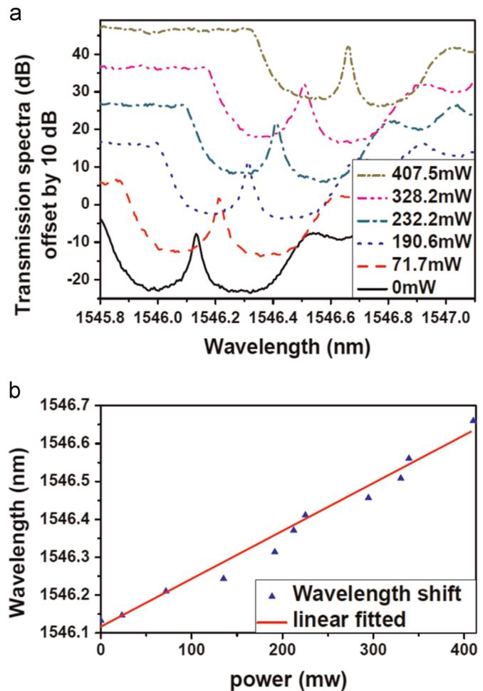
**Fig. 4.** Experiment results. (a) Transmission spectrum shifts with the increasing heating laser power. (b) The relationship of the transmission peak of the tunable fiber F-P filter and the heating power. The red curve is the linear fit. (For interpretation of the references to color in this figure legend, the reader is referred to the web version of this article.)
